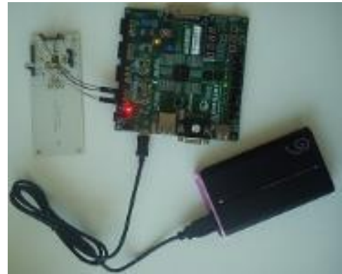
Figure 3. Emulator without microcontroller for application data processing powered with a power bank.
